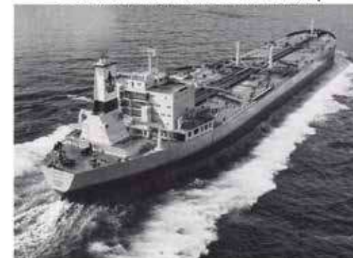
The Hittin is powered by an 8 cylinder, large-bore Burmeister & Wain diesel built at Gotaverken's engine works.
